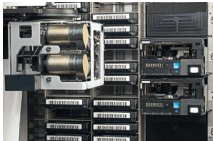
Figure 50: Inside an Automated Tape Library 45
