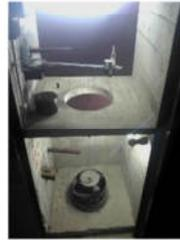
An inverted plumb line is fixed in the rock foundation. Their measurements are translated into absolute horizontal displacements. Information about the sensors that were used and how the measurements were obtained and translated is important for process preservation.
